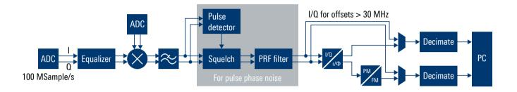
Following decimation and fast Fourier transform of the frequency information, a power spectral density is calculated to obtain the spectral density of frequency fluctuations  $S_{_{\phi}}(f)$ .  $S_{_{\psi}}(f)$  can easily be converted into the spectral density of phase fluctuations  $S_{_{\phi}}(f)$  by dividing by  $f^2$ , where f is the offset frequency from the carrier.
