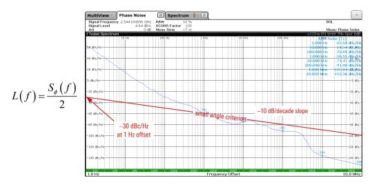
Figure 6. Phase noise measurement showing the confusion resulting from the old definition of phase noise
