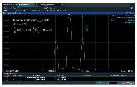
Fig. 3. Spectrum analyzer display of phase modulation where  $\phi_{ok} = 0.01$  rad
