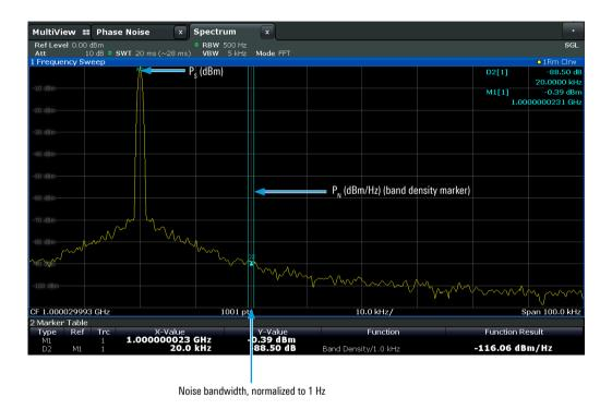
Fig. 1. Direct phase noise measurement using a spectrum analyzer
