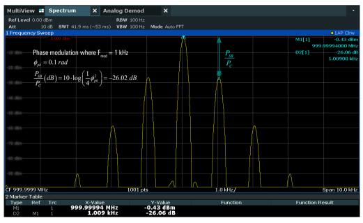
Fig. 4. Spectrum analyzer display of phase modulation where  $\phi_{nk}=0.1\ \text{rad}$
