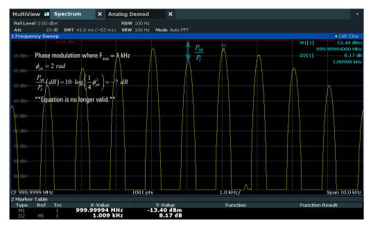
Fig. 5. Spectrum analyzer display of phase modulation where  $\phi_{nk} = 2$  rad
