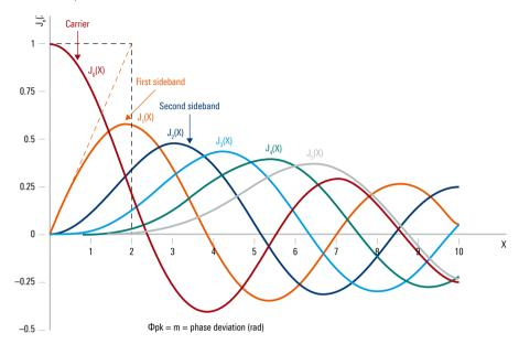
Fig. 2. Bessel functions showing the relationship of sideband voltage to  $\phi_{\text{ok}}$  for phase modulation
